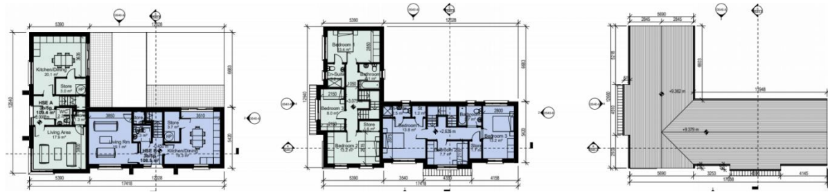
Figure 2.60 Proposed ground (left) first (middle) and roof (right) plans of House Type A-B.
