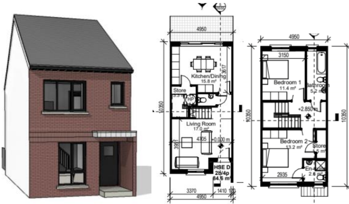
Figure 2.65 Front elevation and Proposed Ground and First Floor Plan of House Type D.
